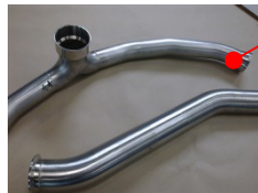
Engine Bleed Ducting
