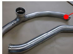
Engine Bleed Ducting
