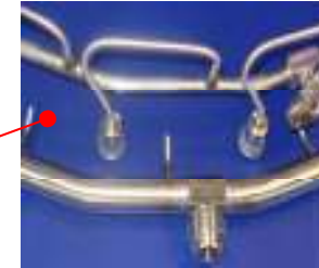
Hydraulic/Fuel Feed Manifolds
