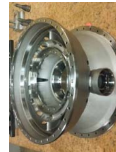
TFE 731 Learjet/Hawker Bearing Support Housing
