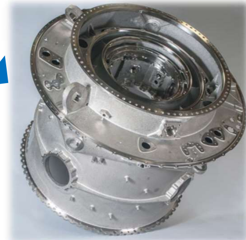
Final product with 7200 close tolerance features
