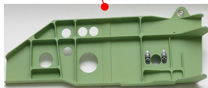
737 Main Landing Gear Wheel Well
