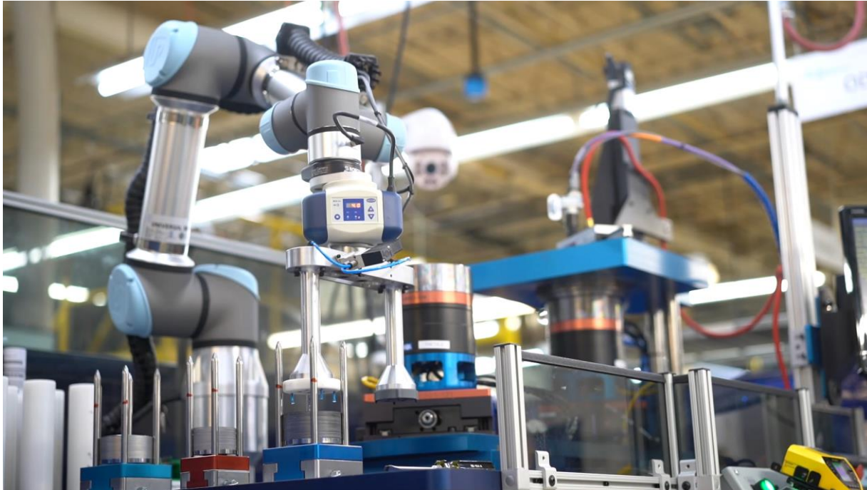
Automated Inner Diameter Bellows Welding
