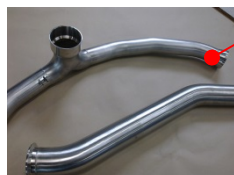
Engine Bleed Ducting
