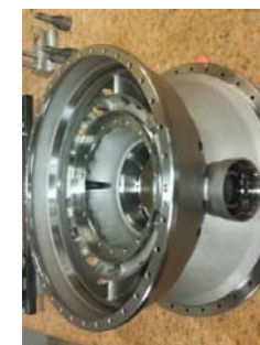
TFE 731 Learjet/Hawker Bearing Support Housing
