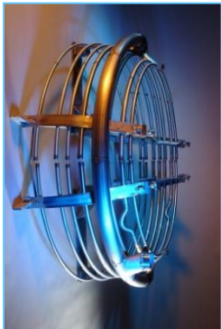
Active Clearance Control System
