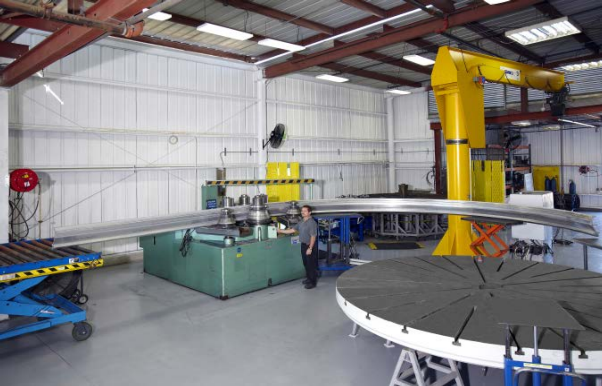
CNC controlled 4-roll rounder & 700 ton expansion, with 800 ton clamp.
