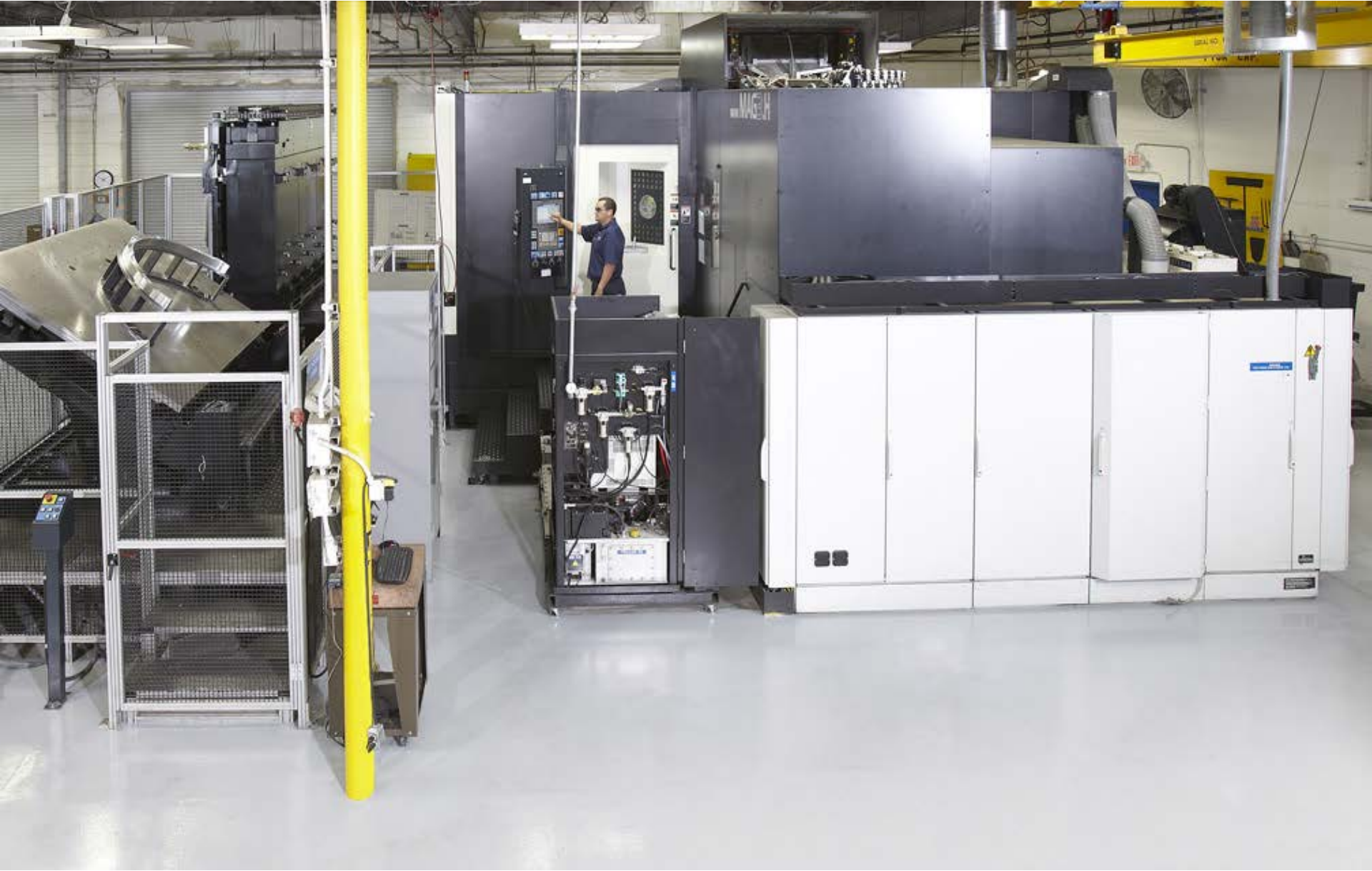
Makino Mag3H, 5-axis 33k rpm, 118" x 72" x 40" working envelope.
