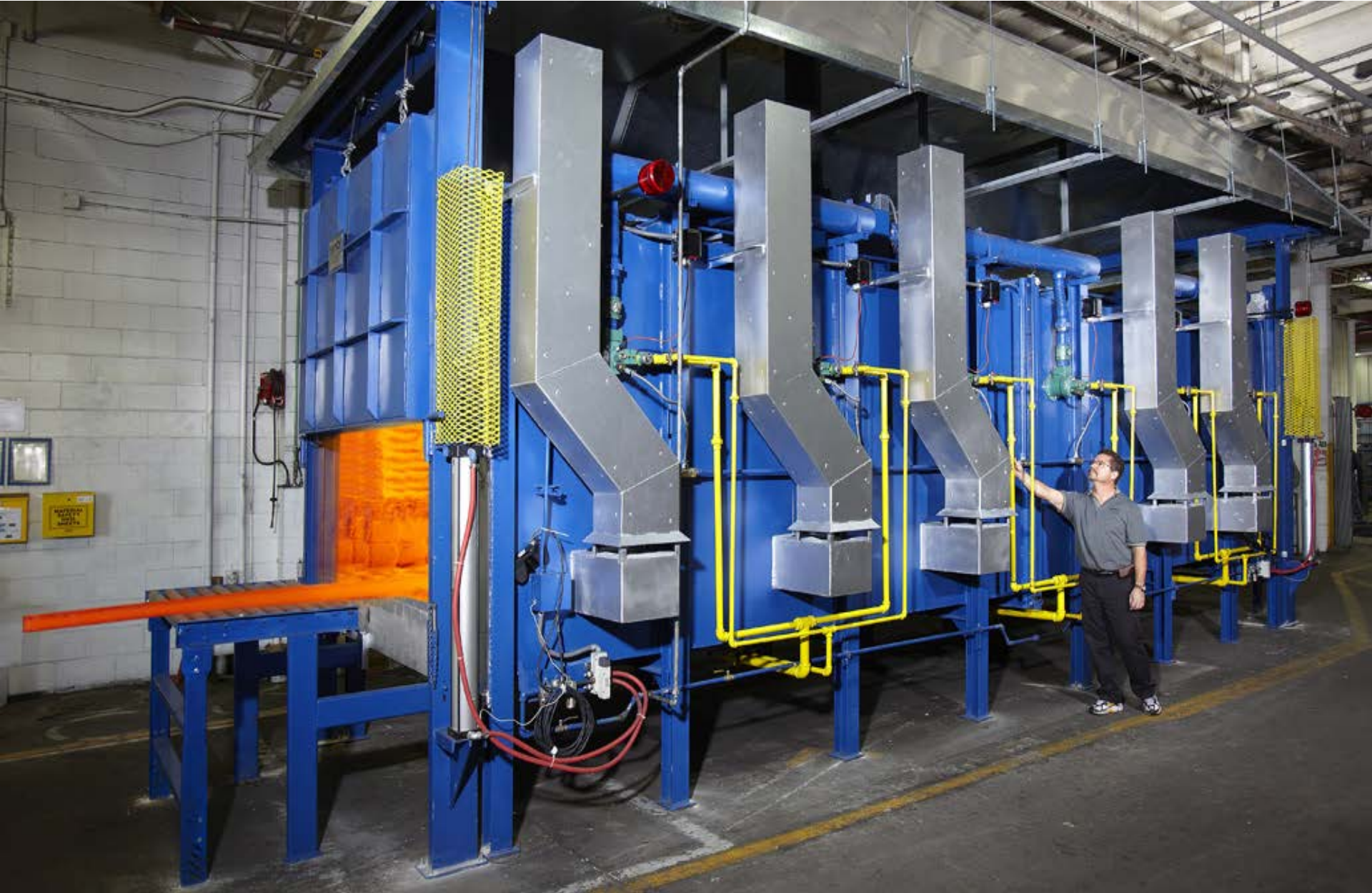
32 ft gas fired forming furnace.
