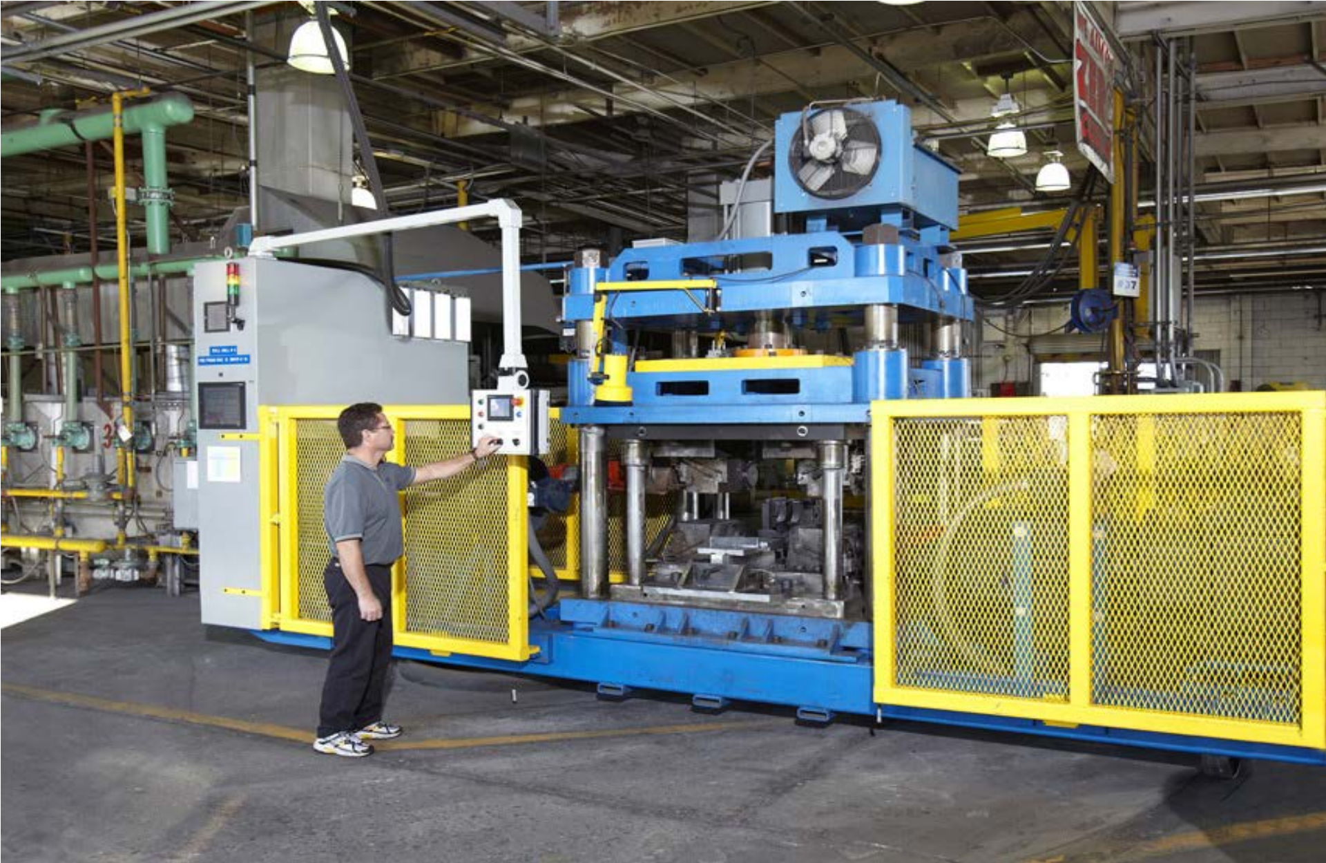
Custom roll-form, 100 ton, CNC controlled.
