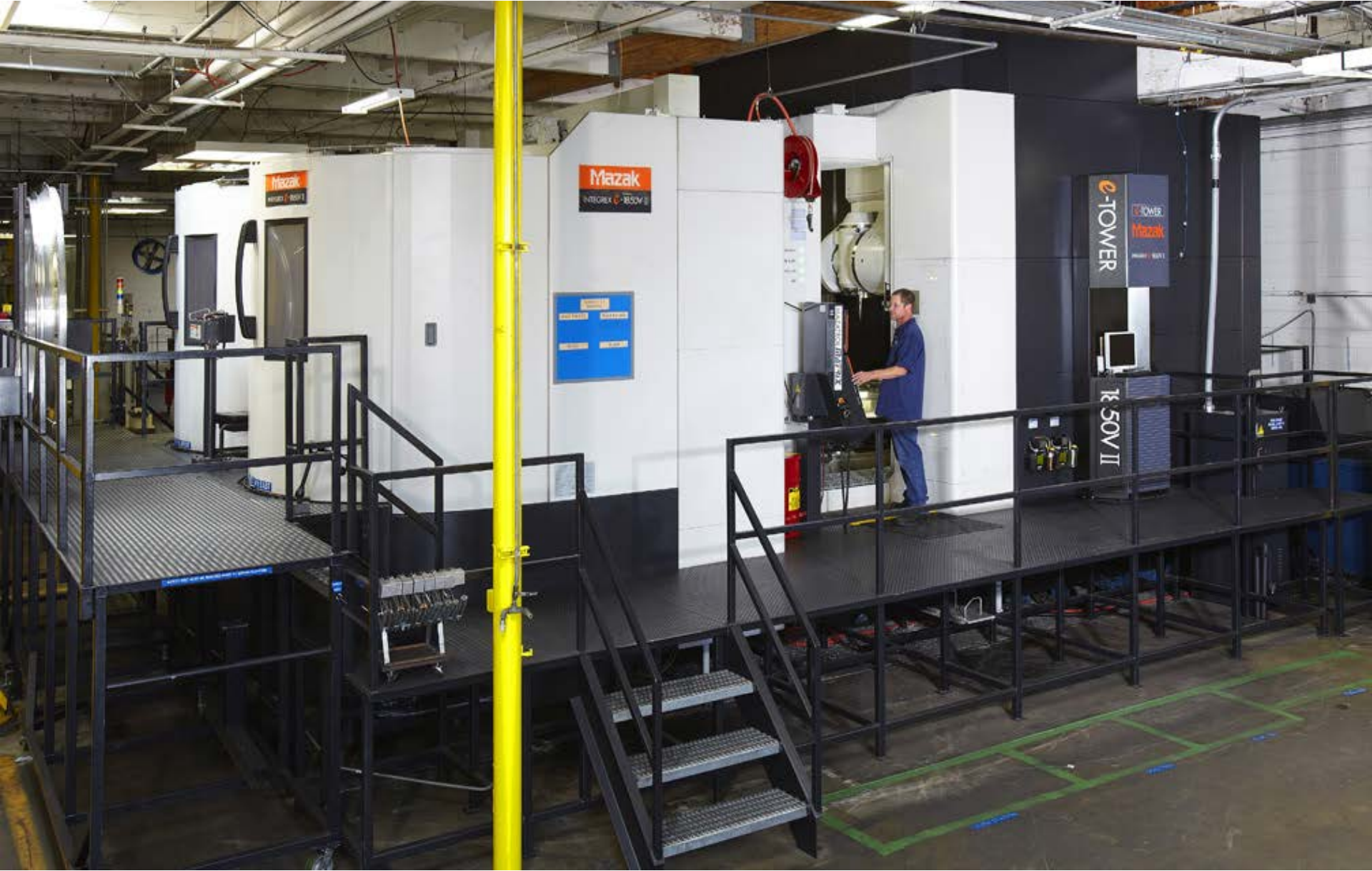
Mazak #1, 10k rpm 5-axis milling w/200 rpm mill-turn table, 92" x 70" working envelope.
