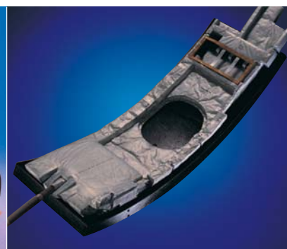
Fuselage insulation panel with integral air distribution ducting
